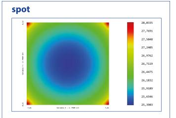
• spot radius in μm at 86% level for a Gaussian laser beam (M<sup>2</sup>=1) with 25 mm diameter at 1/e<sup>2</sup>, clipped at 1/e<sup>2</sup>
